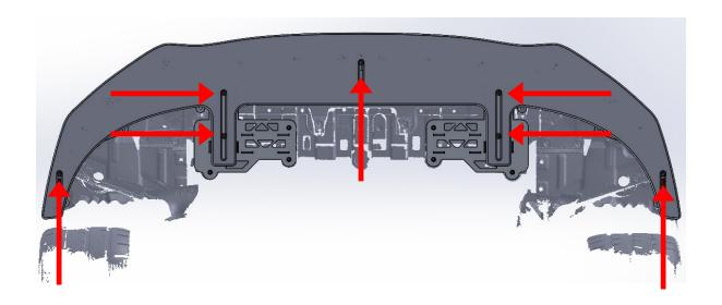
Due to tolerances, there may be a gap between the lip and the splitter board. To rectify this, the splitter board must be removed. After that remove the rear screws from the splitter holder and place the washers supplied between the spacer sleeve and splitter holder and tighten the screws again. Then assemble the splitter board. The gap is now removed
