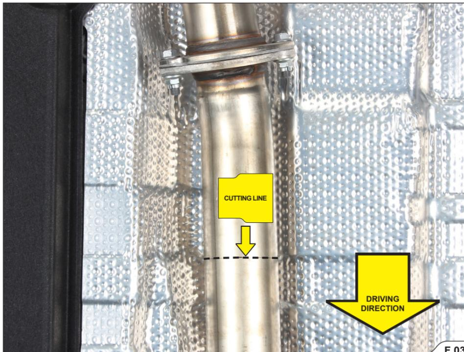
2. Support the exhaust system, undo all marked rubber brackets and carefully remove the exhaust system off the vehicle (F 04, 05, 06, 07).
